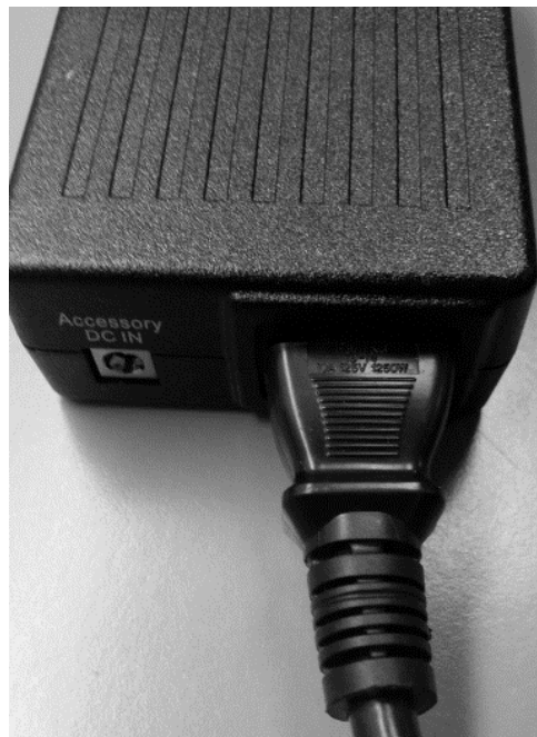
Figure 6.2: Connecting AC Cable to Power Supply
