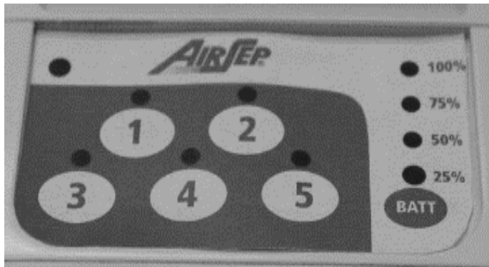
Figure 23.2: Adhering New Control Panel
