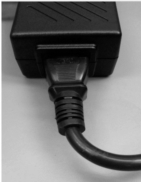
Figure 7.2: Connecting AC Cable to Power Supply
